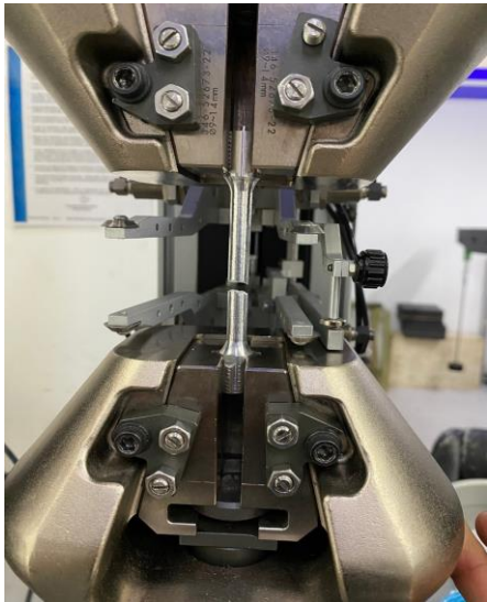
Imagen 3. Item at rupture. Image 3. Item at break.
